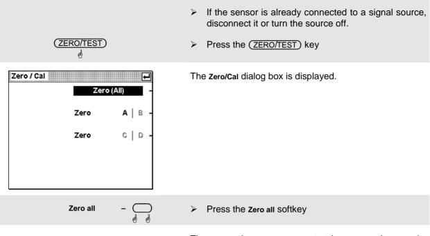
The correction measurement takes several seconds. When completed a GO/NOGO message is output.
