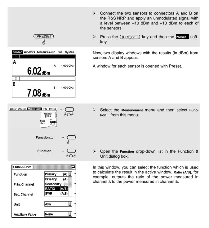
> Check whether Sensor A is selected in the drop-down list for the primary channel and Sensor B in the dropdown list for the secondary channel.
